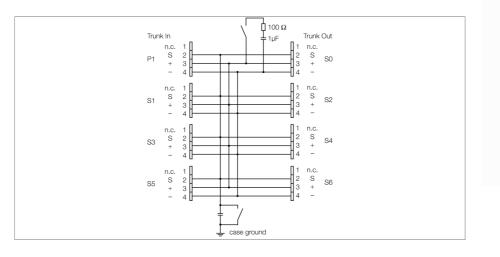
The 6-channel junction box JBBS-48-T615/3G is designed for PROFIBUS-PA systems.
