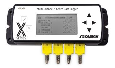
The OM-CP-QUADTCTEMP2000-A2 and OM-CP-OCTTCTEMP2000-A2 are four and eight channel thermocouple data loggers with an LCD screen. The device features on-screen minimum, maximum and average statistics, as well as a user configurable screen that allows for any combination of channels to be displayed. The device accepts J, K, T, E, R, S, B and N type thermocouples.
