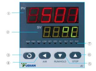
① Indicator lamps: OP1 and OP2 indicate the status of current retransmission. AL1, AL2, AU1and AU2 indicate the I/O actions of the corresponding modules.
