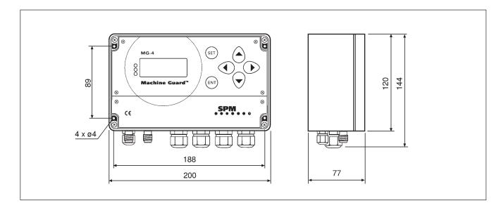
Machine Guard MG4-12A is a stand-alone measuring unit for continuous monitoring of machine vibration (one channel) and bearing condition (two channels). It measures vibration severity (true RMS value of vibration velocity) according to ISO 10816 and shock pulses according to the true SPM method.
