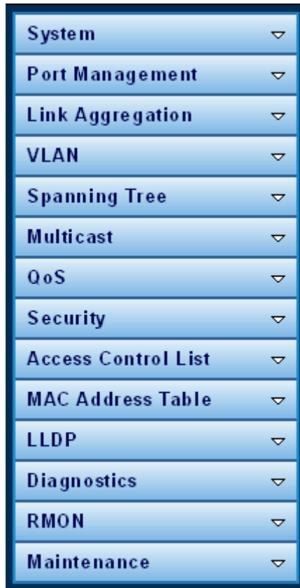
Figure 4-1-5 Managed Switch Main Functions Menu
