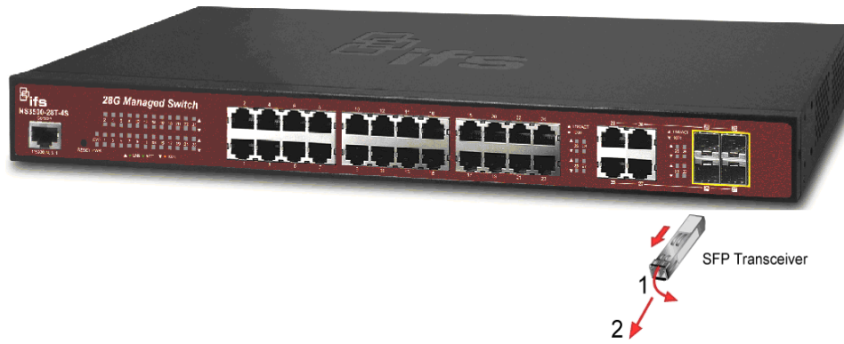
Figure 2-1-8 How to Pull Out the SFP Transceiver
