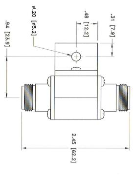
1.5 to 50MHz @ 2kW 50 to 220MHz @ 375W 220 to 400MHz @ 125W IPOYPICISE!
