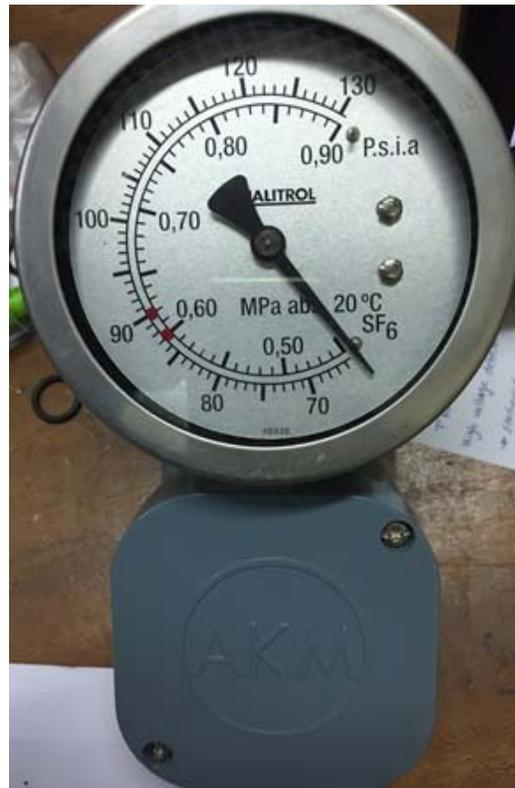
**Part No. & Model of SF6 Gas Density Monitor**
