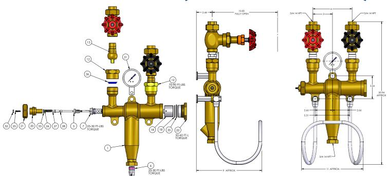
NOTE: A strainer and steam trap is recommended to be used in conjunction with all our steam mixing units. Foreign deposits in supply lines can effect ball check durabilility. Proper steam and water treament is recommended to ensure proper performance and durability. Unit should be shut-off when not in use for extended periods of time.
